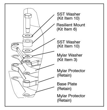
Figure 6-8 Compressor Lower Mounting
