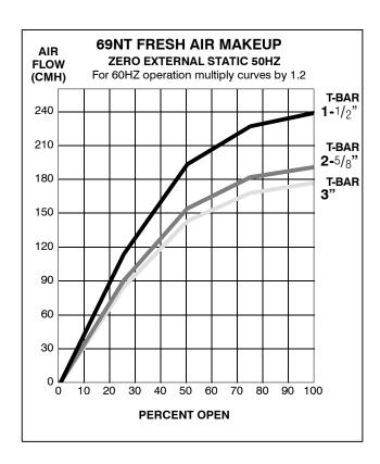
Figure 4-1 Make Up Air Flow Chart
