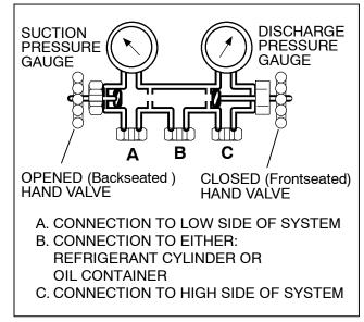
Figure 6-3 Manifold Gauge Set
