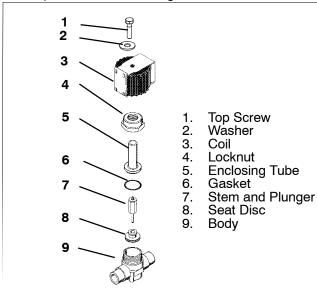
Figure 6-14 Unloader Solenoid Valve
