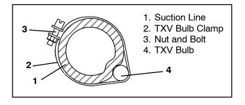
Figure 6-10 Thermostatic Expansion Valve Bulb
