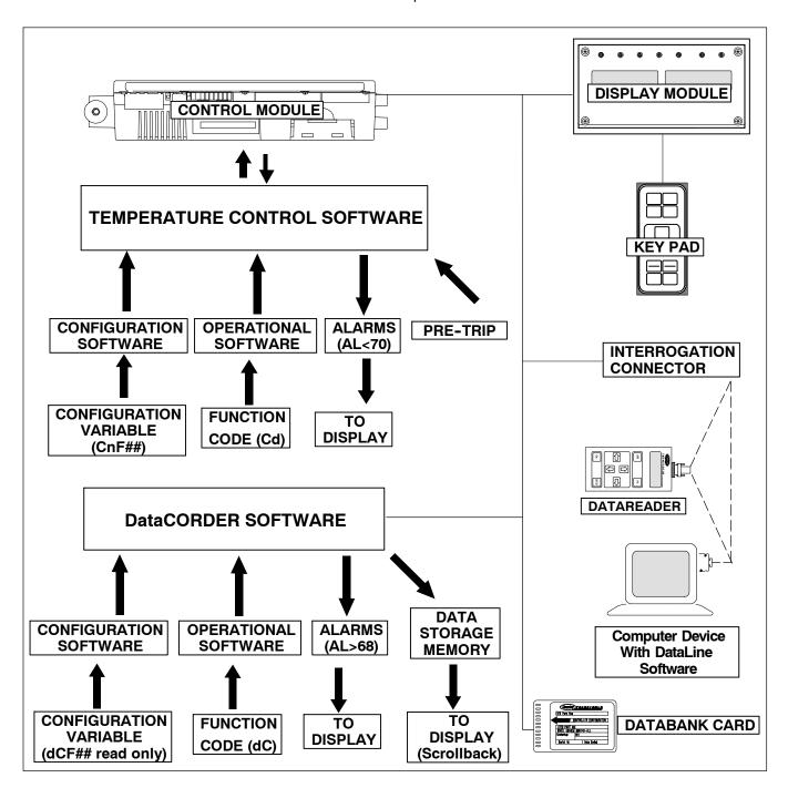
Figure 3-1 Temperature Control System
