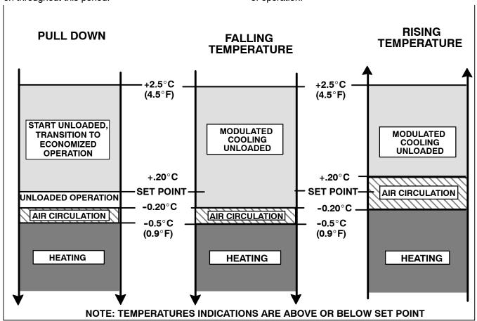
Figure 4-2 Controller Operation - Perishable Mode
