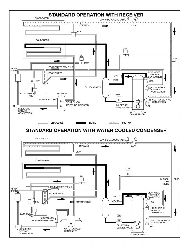
Figure 2-6 Refrigeration Circuit Schematic - Standard Operation
