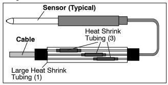
Figure 6-20 Typical Sensor and Cable Splice
