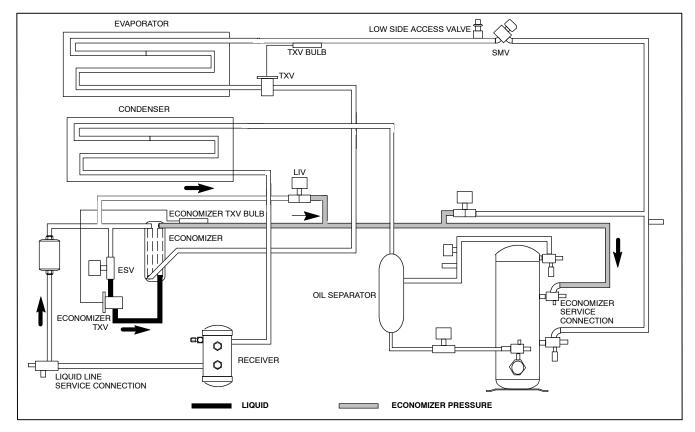
Figure 2-7 Refrigeration Circuit Schematic - Economized Operation
