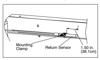
Figure 6-22 Return Sensor Positioning
