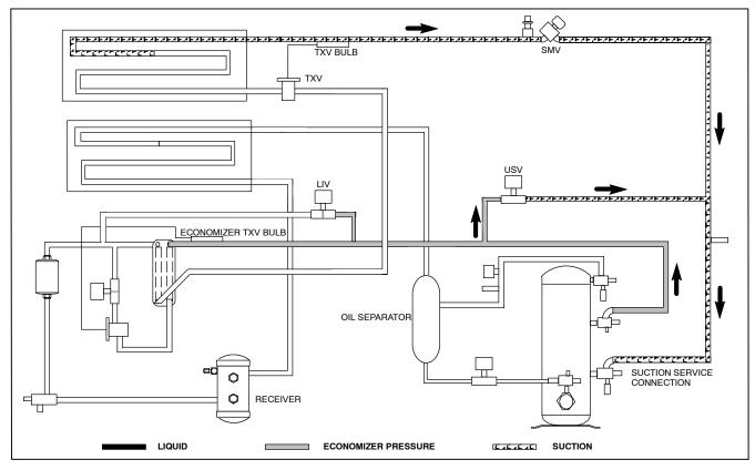
Figure 2-8 Refrigeration Circuit Schematic - Unloaded Operation
