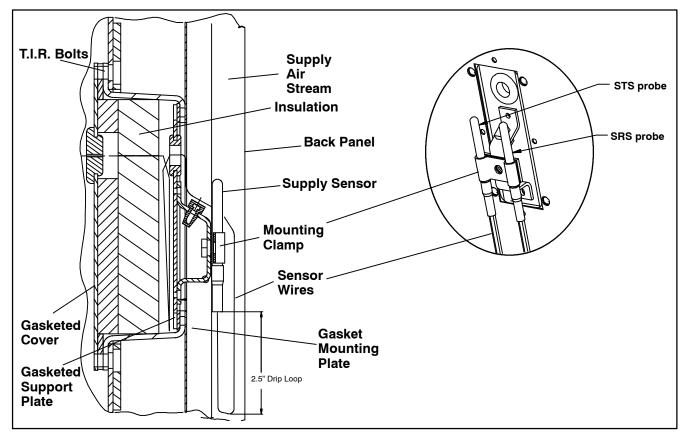
Figure 6-21 Supply Sensor Positioning
