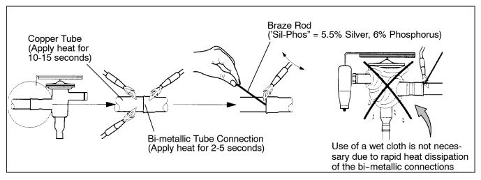
Figure 6-13 Hermetic Thermostatic Expansion Valve Brazing Procedure
