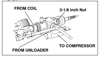
Figure 6-17 Suction Modulation Valve (SMV)
