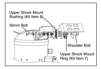
Figure 6-7 Compressor Upper Mounting
