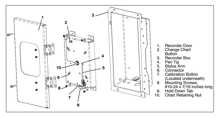
Figure 6-23 Electronic Partlow Temperature Recorder
