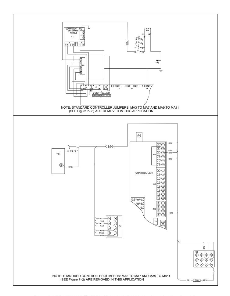
Figure 7-3 SCHEMATIC DIAGRAM, WIRING DIAGRAM- Electronic Partlow Recorder
