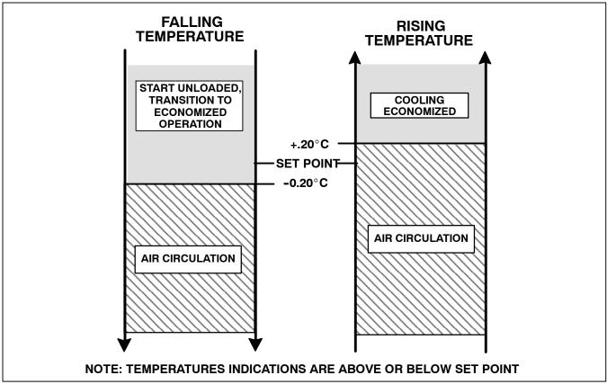
Figure 4-3 Controller Operation - Frozen Mode
