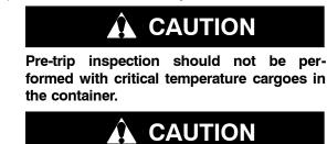
When Pre-Trip key is pressed, economy, dehumidification and bulb mode will be deactivated. At the completion of Pre-Trip activity, economy, dehumidification and bulb mode must be reactivated.
