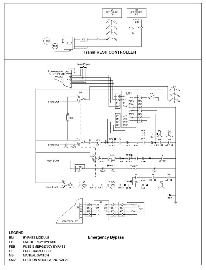
Figure 7-6 SCHEMATIC DIAGRAM-TransFRESH and Emergency Bypass (For Single Phase Evaporator Fan Motor Applications)
