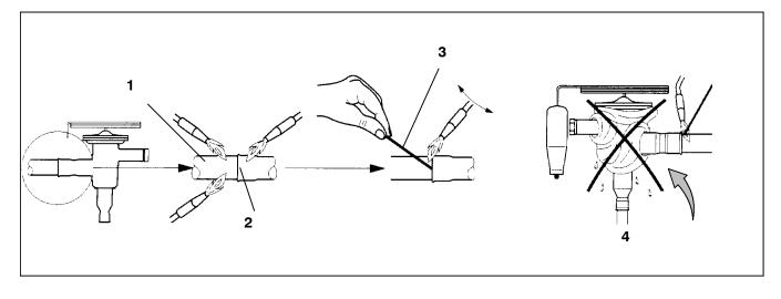
1. Copper Tube (Apply heat for 10-15 seconds)
