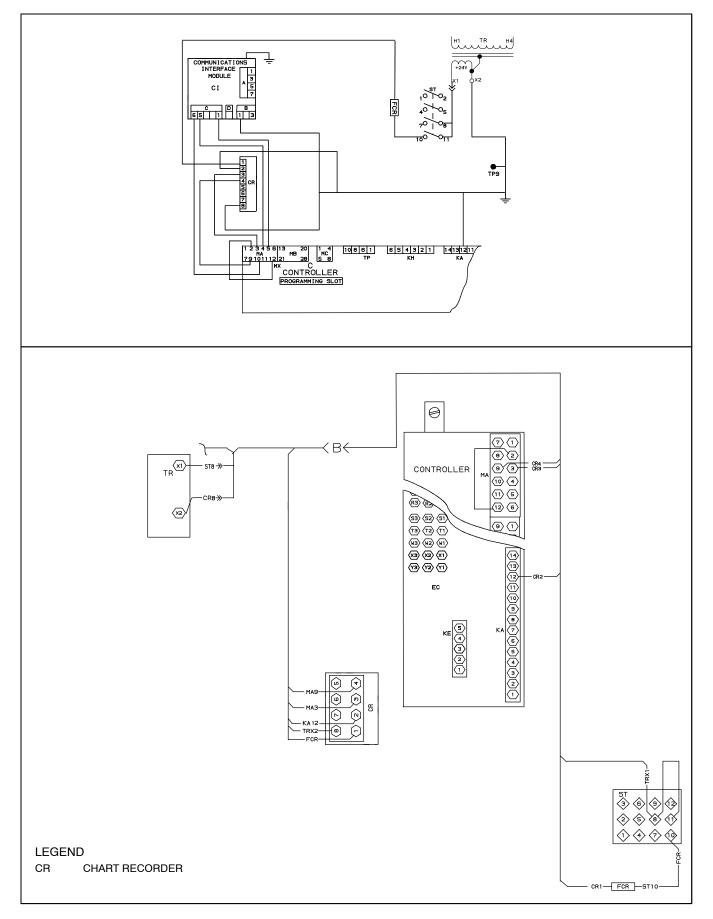
Figure 7-7 SCHEMATIC AND WIRING DIAGRAM - Electronic Partlow Recorder (For Single Phase Evaporator Fan Motor Applications)
