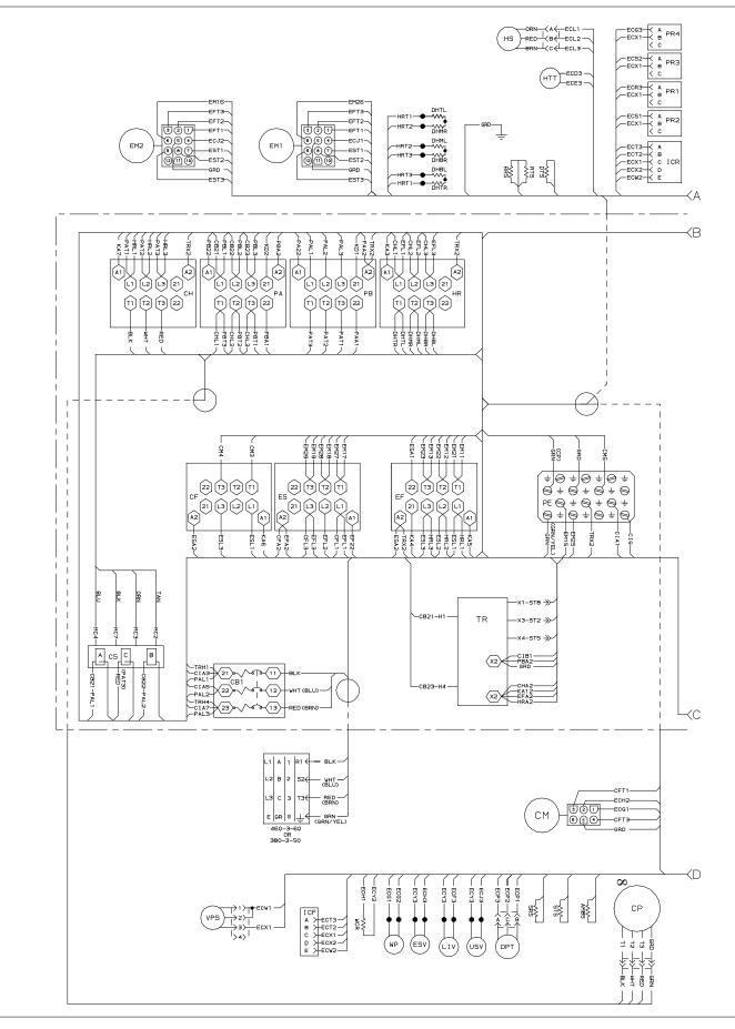
Figure 7-12 WIRING DIAGRAM - Three-Phase Evaporator Fan Motor (Sheet 1 of 2)
