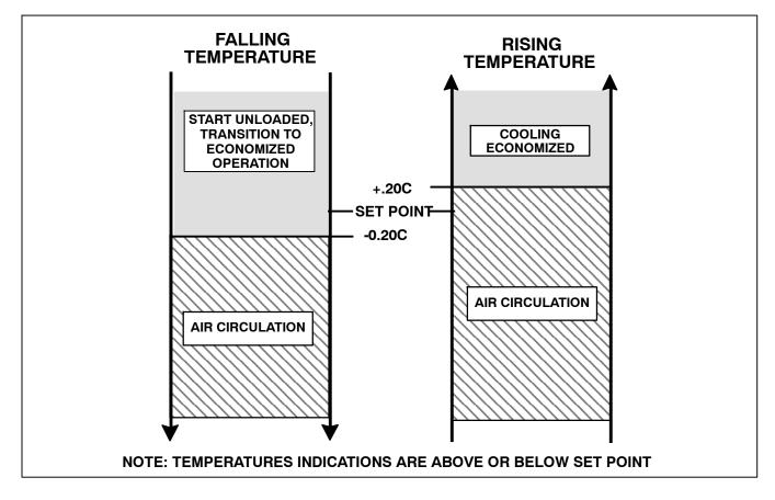
Figure 4-4 Controller Operation - Frozen Mode
