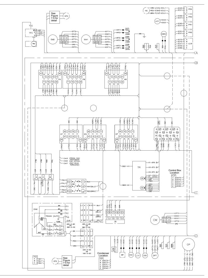
Figure 7-9 WIRING DIAGRAM - Single Phase, Normal Evaporator Fan Capability (Sheet 1 of 2)
