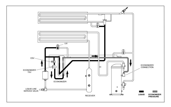
Figure 2-8 Refrigeration Circuit Schematic - Economized Operation
