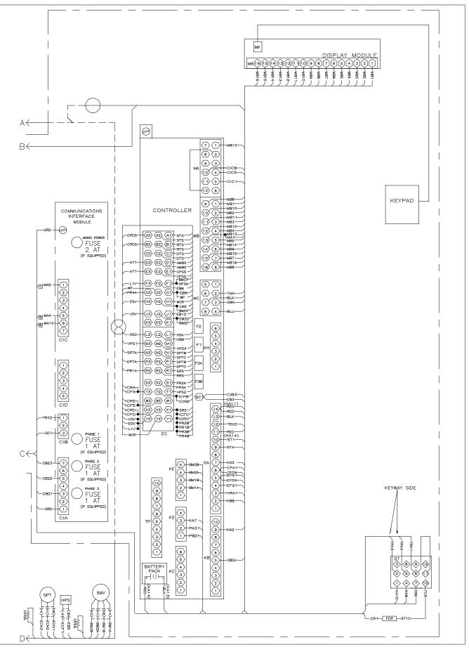
Figure 7-10 WIRING DIAGRAM - Normal Evaporator Fan Capability with Bypass Module (Sheet 2 of 2)
