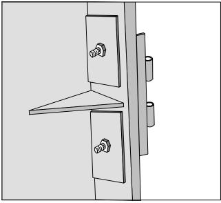
Figure 6-25 Door Hinge Repair
