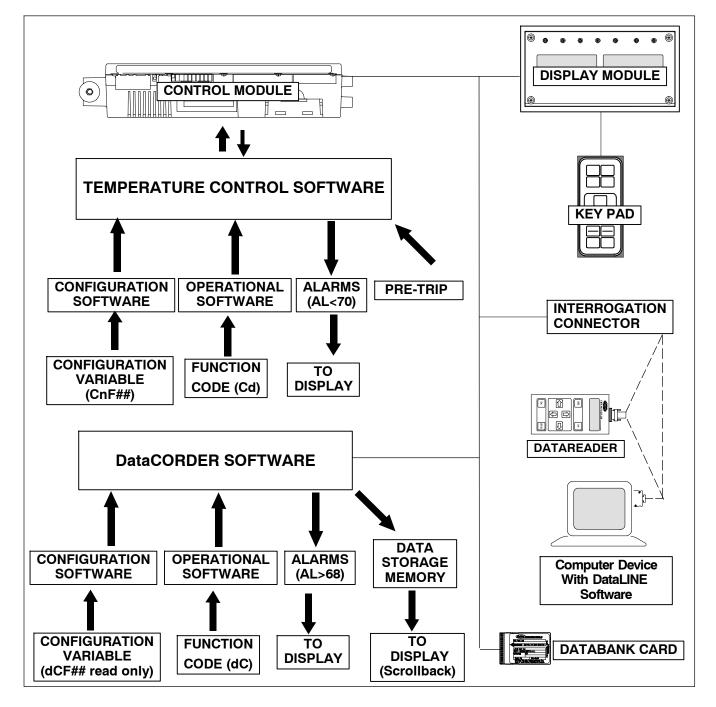
Figure 3-1 Temperature Control System
