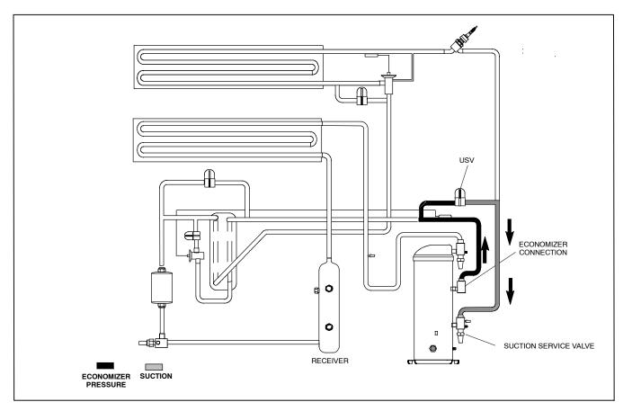
Figure 2-9 Refrigeration Circuit Schematic - Unloaded Operation
