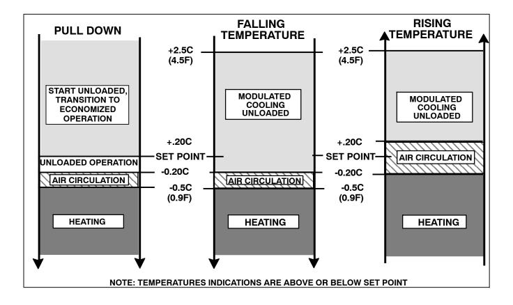
Figure 4-3 Controller Operation - Perishable Mode
