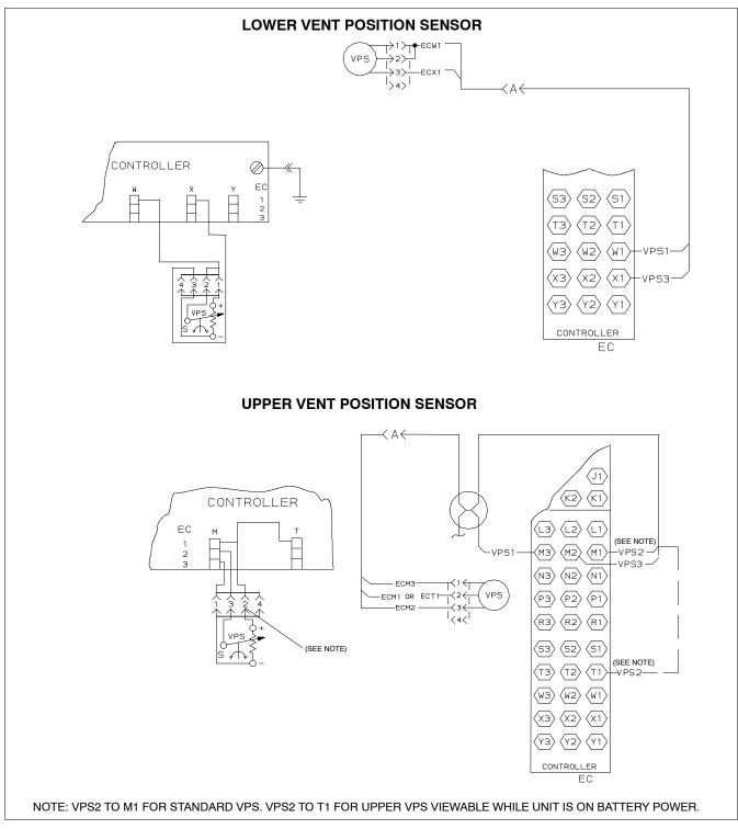
Figure 7-8 SCHEMATIC AND WIRING DIAGRAM - Upper and Lower Vent Position Sensors
