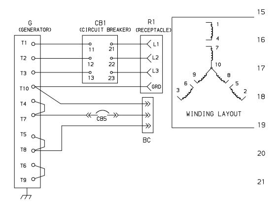
FIGURE 4.7 ELECTRICAL WIRING SCHEMATIC - DRAWING NUMBER 62-11257-00 REV - HIGH VOLATGE INFORMATION (PID RG1160 ONLY)
