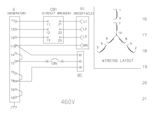
FIGURE 4.4 ELECTRICAL WIRING SCHEMATIC - DRAWING NUMBER 62-10386-00 REV - HIGH VOLATGE INFORMATION (PID RG0466 ONLY)
