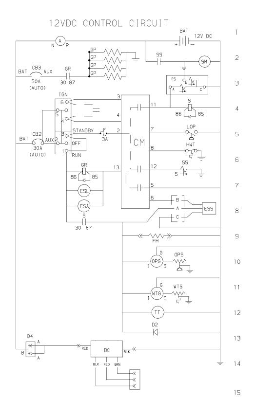
FIGURE 4.3 ELECTRICAL WIRING SCHEMATIC - DRAWING NUMBER 62-10386-00 REV - (PID RG0466 ONLY)
