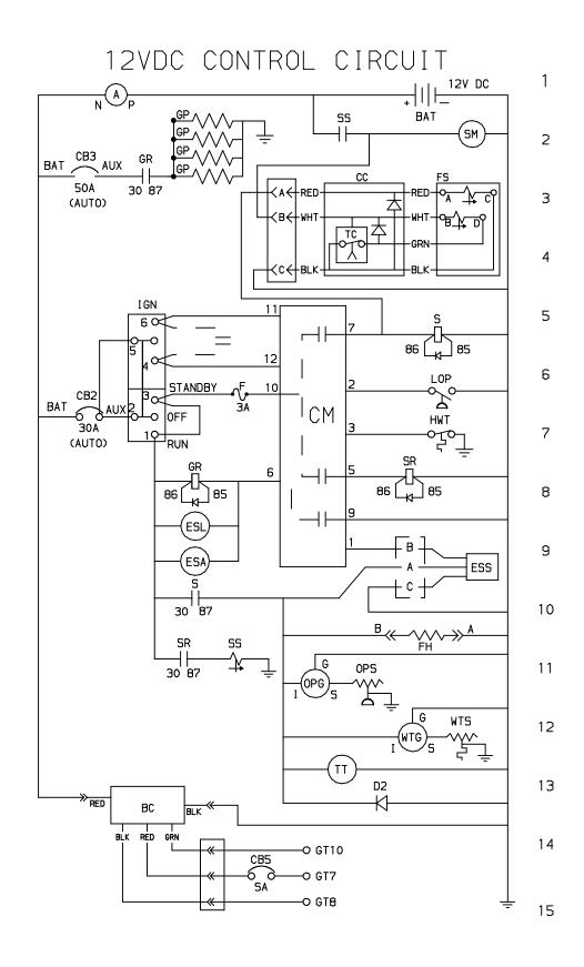
FIGURE 4.6 ELECTRICAL WIRING SCHEMATIC - DRAWING NUMBER 62-11257-00 REV - (PID RG1160 ONLY)
