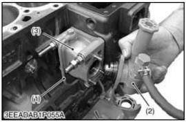
1. Oil Pipe3. Fuel Feed Pump2. Fuel Feed PumpHolder
