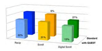
While energy costs can be improved up to 27% moving from reciprocating compressor technology to today's digital scroll units, the savings when QUEST is added are even greater.
