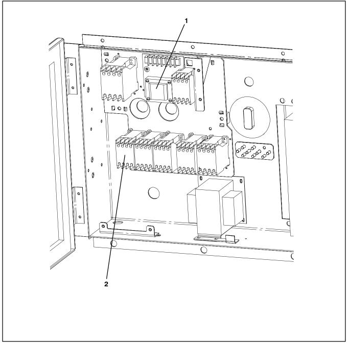
1. Humidity Power Transformer (HPT) with Fuse (FH) for Humidity Water Pump (HWP)
