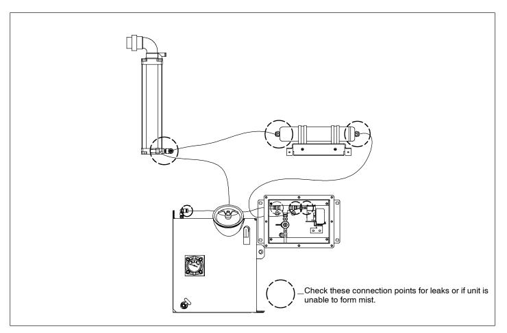
**Figure 6-1 Humidity System Connection Points**
