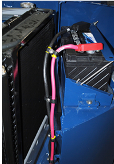
Figure 5.2 Battery Cable Routing - Side View
