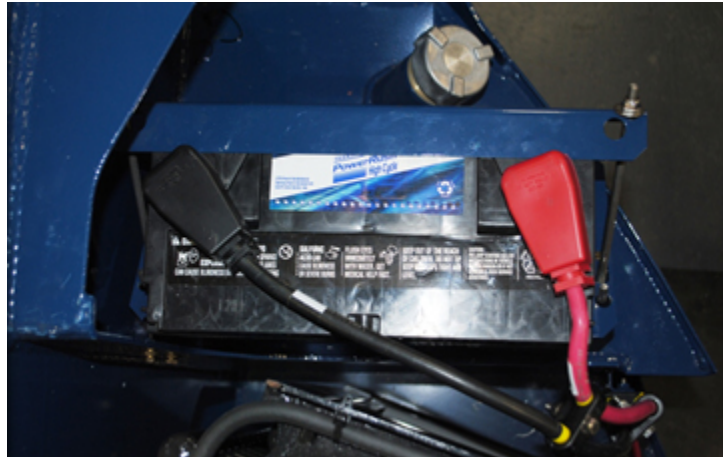
Figure 5.2 Battery Cable Routing - Side View
