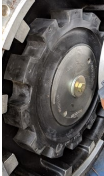
Figure 5.7 Generator Coupler Bolt
